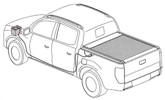
电源线直接接入汽车电瓶 The power cord is directly connected to the car battery.
