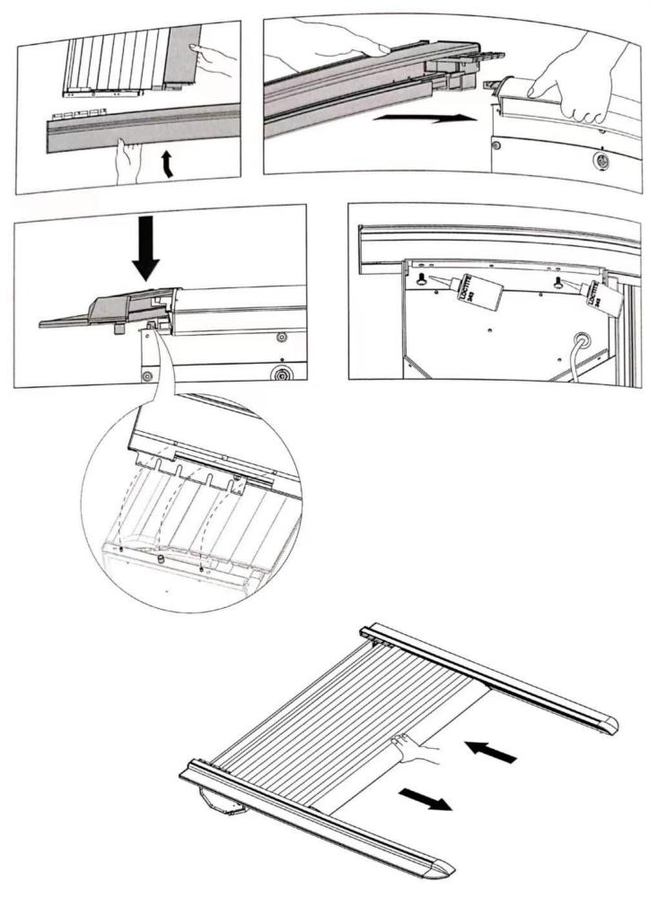
前后推拉卷帘以确保卷帘能顺畅地滑动 Push and pull the tonneau cover back and forth to ensure that the tonneau cover can slide smoothly
