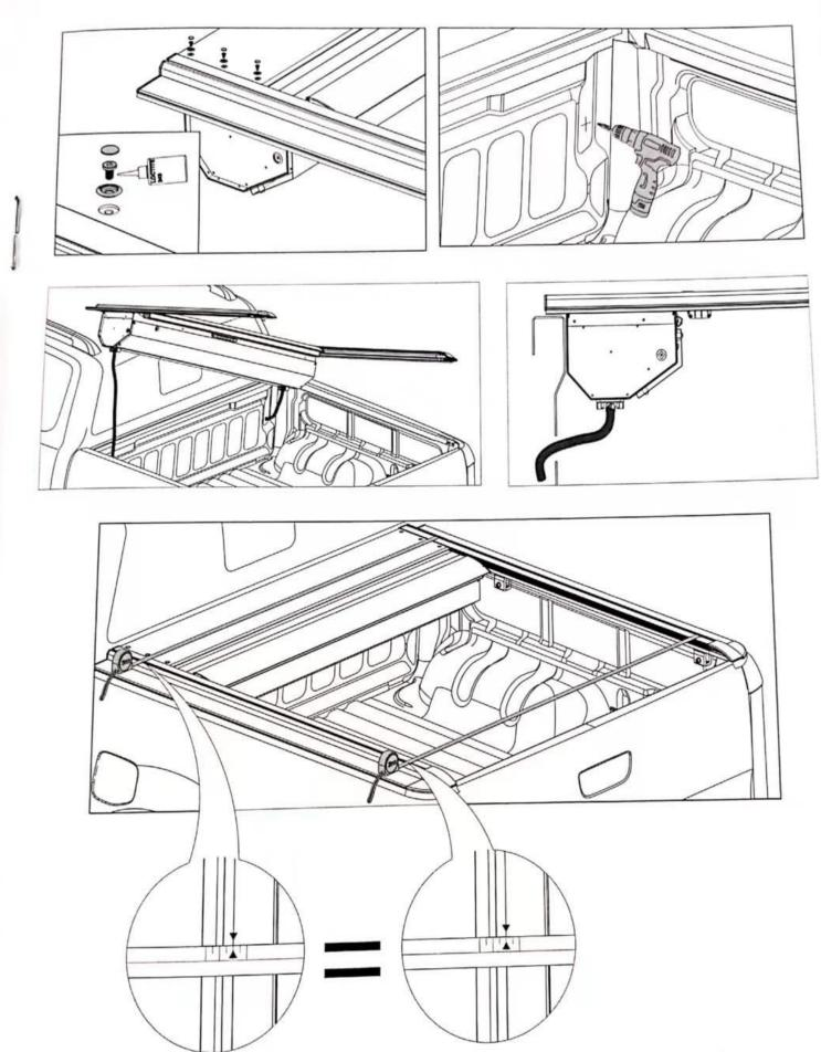
调整卷帘前后两端的宽度,要使前后两端的宽度一致 Adjust the width of the front and rear ends of the tonneau cover to make the width of the front and rear ends the same.
