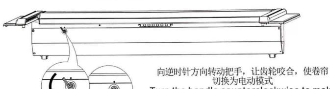
Turn the handle counterclockwise to make the gear engage, so as to switch the tonneau cover to the electric mode.
